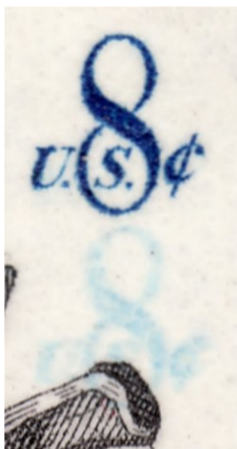
Ghost impression due to contaminated rollers during taggant application.
